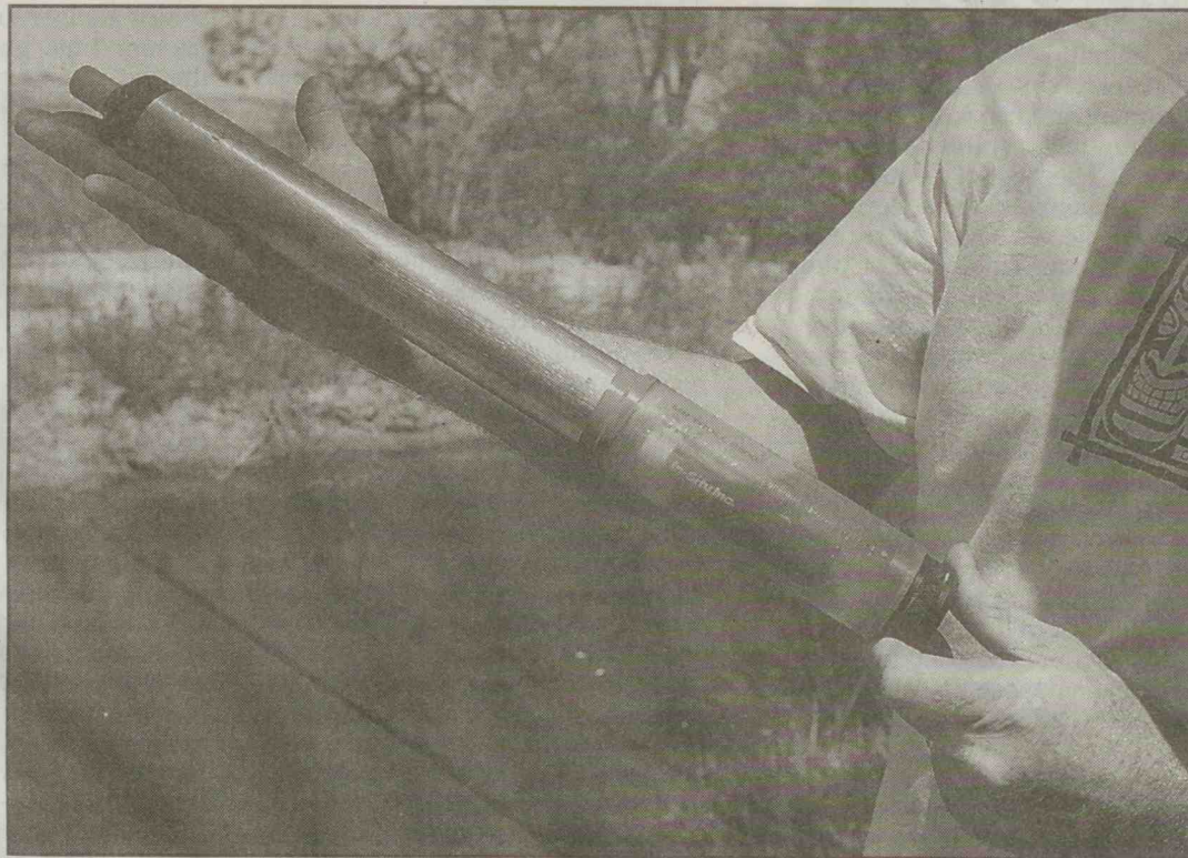
Scientists will place this probe and others into the San Diego River at various points to help monitor water conditions and provide a range of data for their studies. Earnie Grafton / U-T
